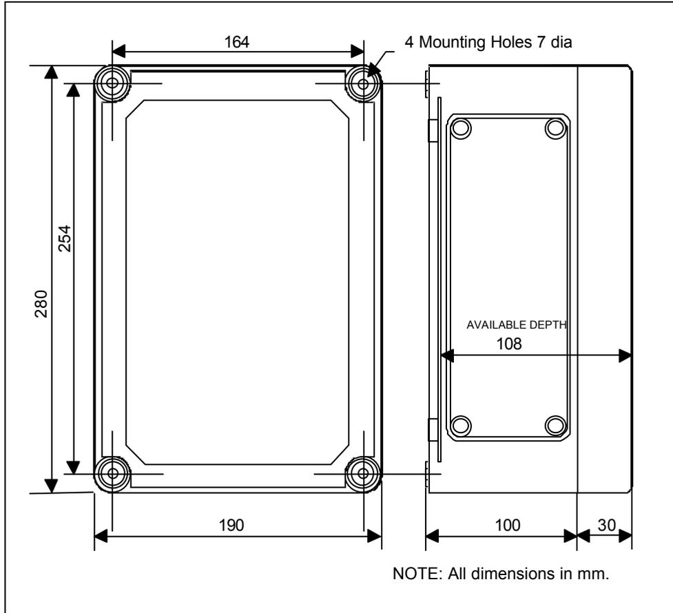
The Basic Enclosure is an impact resistant, polycarbonate enclosure which offers protection from dust and moisture in accordance with IP67 (IEC529/DIN 40050/BS5490). It is moulded from homogeneous thermoplastic polycarbonate, is resistant to normal atmosphere corrosion and is resistant to most mineral and organic acids. Contact should be avoided, however, with organic solvents and strong alkalis. The material is self-extinguishing and does not release any toxic combustion products.
